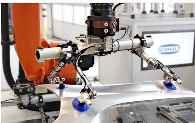
Pipe SXT-RT for assembling a complete tooling for handling formed car body parts
