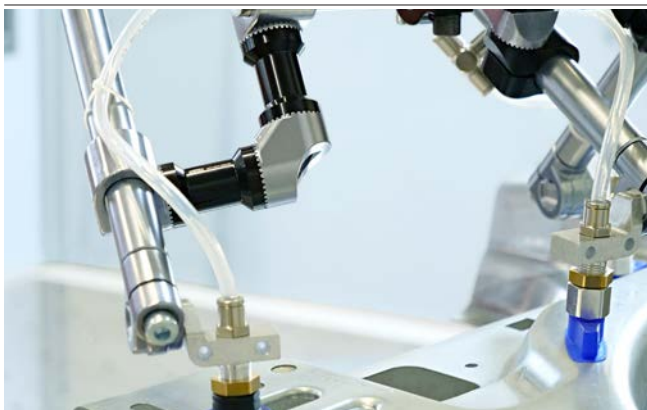
Truss connector (geared) SXT-TC in combination with holder HT-SG and suction cup SAX when handling an automotive part
