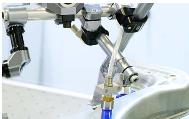
Elbow connector (geared) SXT-ANG when handling a formed sheet metal part
