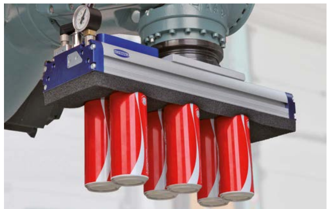
Vacuum area gripping system FXP being used to handle beverage cans
