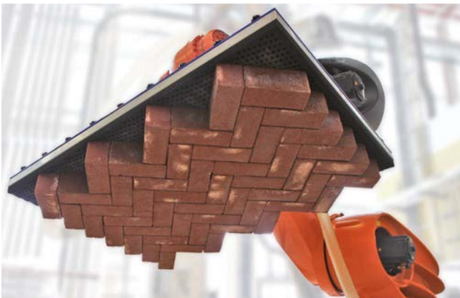
Construction materials | Vacuum layer gripping system SPZ being used to handle clinker bricks
