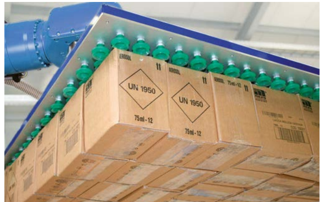
SPZ Packaging | Palletizing and de-palletizing of cardboard boxes, beverage trays etc.
