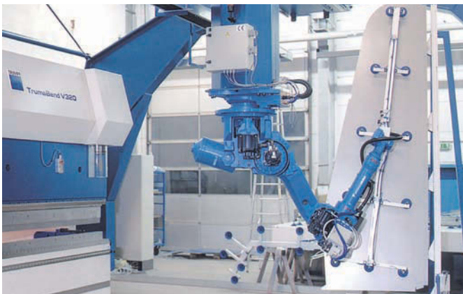
Car body construction | Vacuum suction spider SSP for the machine loading and unloading of metal sheet cuts in the agricultural machinery car body manufacturing
