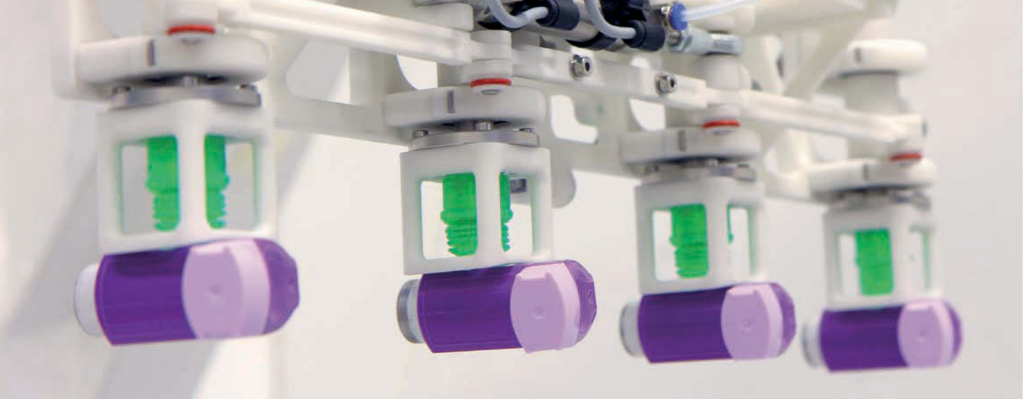
Pharma | Generative manufactured High-Speed-Picker with rotary modules for the handling of medical products
