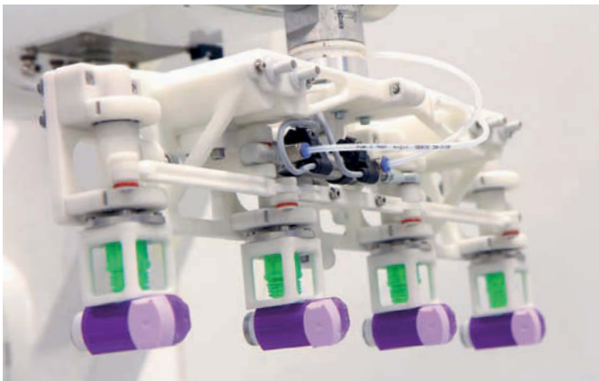
The High-Speed-Picker functions with individual vacuum absorption circuits
