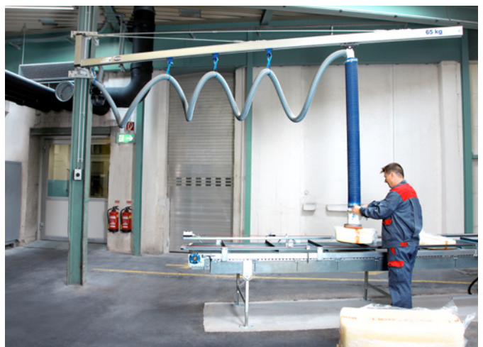
Aluminum wall mounted jib crane, mounted to a production hall pillar, with vacuum tube lifter JumboSprint during handling of raw rubber bales
