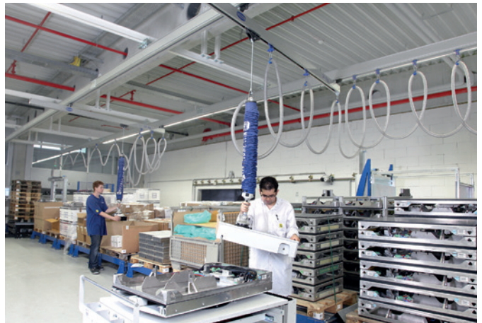
Aluminum crane system SRA with vacuum tube lifter Jumbo
