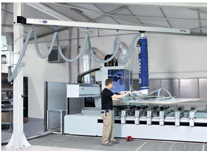
Aluminum column mounted jib crane with vacuum tube lifter JumboErgo during loading of a CNC machining center
