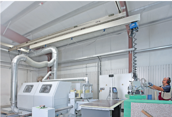
Aluminum single bridge crane system with telescopic jib and vacuum lifting device VacuMaster Comfort handling plastic sheets
