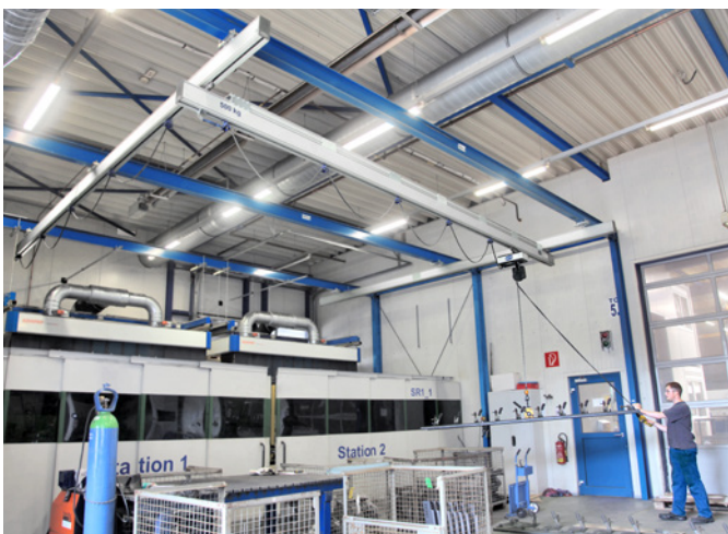
Aluminum single bridge crane system with reinforced section and chain hoist during machine loading
