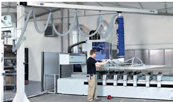
Complete handling system with vacuum tube lifter Jumbo and crane
