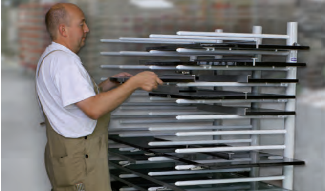
Transport trolley HW for storing and transporting workpieces
