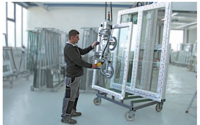
Vacuum lifting VacuMaster Window device being used for picking windows with plastic frames
