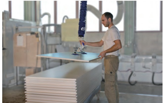
Vacuum tube lifter JumboFlex for handling light, coated wooden boards up to 50 kg
