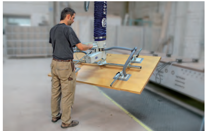
Vacuum tube lifter JumboErgo with pneumatic swiveling unit PSE for swiveling workpieces by 90°
