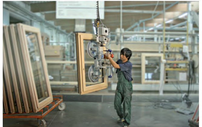
Vacuum lifting device VacuMaster Window being used to unload a vertical glazing press
