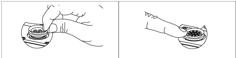
Remove and insert the seal of the electric feed-through module
