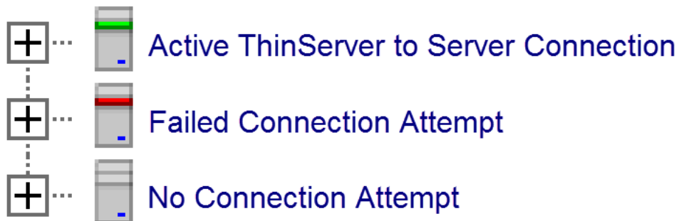
Terminal Server Status Lights
