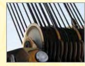
Encoder tracks rotations of a drum used to store cable.
