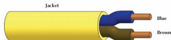
Typical AS-i cable
