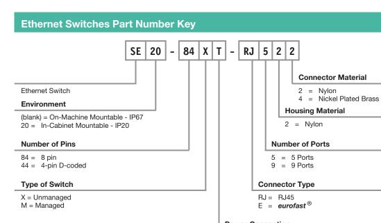
**Power Connection** (blank) = 5 pin *minifast* ® 4 = 4 pin *minifast*<sup>®</sup> T = Terminal Strip
