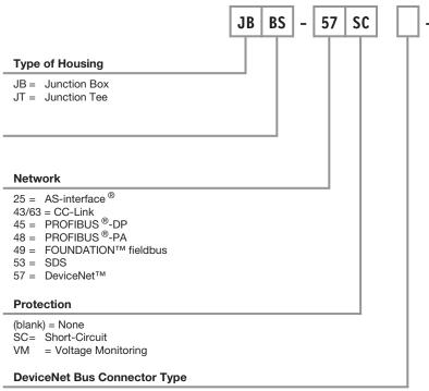
(Blank) = minifast Bus Connectors FS = Male M12 Bus Connectors FS/VM = Male M12 Bus Connector with Voltage Monitoring
