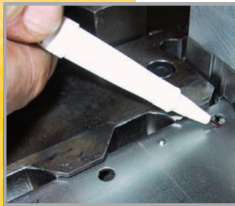
Inductive proximity sensor used for strip feed, N.O. switch
