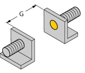
The given minimum distances have been checked against the standard switching distance. Should the sensitivity of the sensors be changed via potentiometer, the data sheet specifications no longer apply.
