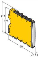
7580020 Isolating switching amplifier, 2channel; SIL2 acc. to IEC 61508; Ex-proof version; 2 transistor outputs; input Namur signal; ON/OFF switchable monitoring of wire-break and short-circuit; toggle between NO/ NC mode; signal doubling; removable screw terminals; 12.5 mm wide; 24 VDC power supply
