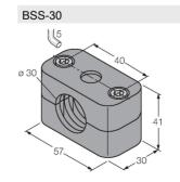
6901319 Mounting clamp for smooth and threaded barrel sensors; material: Polypropylene
