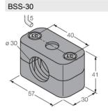
Mounting clamp for smooth and threaded barrel sensors; material: Polypropylene
