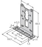
6945006 Mounting bracket for rectangular Q14 or Q20; material VA 1.4301
