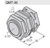
Quick-mount bracket with dead-stop; material: brass, PTFE-coated; Male thread M36 × 1.5. Note: The switching distance of the proximity switches may change when using quick-mount brackets.
