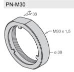
Protective nut for M30 x 1 threaded barrel devices; material: Stainless steel A2 1.4305 (AISI 303)
