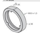
Protective nut for M30 x 1 threaded barrel devices; material: Stainless steel A2 1.4305 (AISI 303) QM-30
