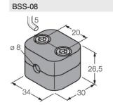
Mounting clamp for smooth and threaded barrel sensors; material: Polypropylene
