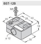
6947212 Mounting clamp for threaded barrel sensors, with dead-stop; material: PA6
