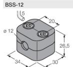
6901321 Mounting clamp for smooth and threaded barrel sensors; material:
