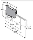
4 digital inputs acc. to EN 60947-5-6 For NAMUR sensors, de-energized contacts or uprox®+ 2-wire DC sensors.
