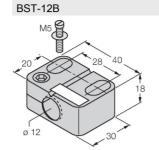
6947212 Mounting clamp for threaded barrel
