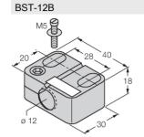
Mounting clamp for threaded barrel sensors, with dead-stop; material: PA6
