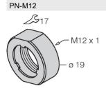
Impact protection nut for M12x1 threaded barrel devices; material: Stainless steel A2 1.4305 (AISI 303)
