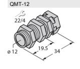
Quick-mount bracket with dead-stop; material: brass, PTFE-coated; Male thread M16 × 1. Note: The switching distance of the proximity switches may change when using quick-mount brackets.
