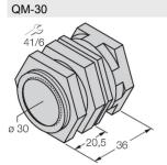
Quick-mount bracket with dead-stop; material: Chrome-plated brass. Male thread M36 × 1.5. Note: The switching distance of the proximity switches may change when using quick-mount brackets.
