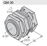
Quick-mount bracket with dead-stop; material: Chrome-plated brass. Male thread M36 × 1.5. Note: The switching distance of the proximity switches may change when using quick-mount brackets.
