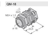
Quick-mount bracket with dead-stop; material: Chrome-plated brass. Male thread M24 × 1.5. Note: The switching distance of the proximity switches may change when using quick-mount brackets.
