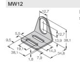
6945003 Mounting bracket for threaded barrel sensors; material: Stainless steel A2 1.4301 (AISI 304)
