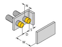
All non-flush mountable *uprox*®+ threaded barrel sensors can be screwed in up to the top edge of the barrel. In this mounting position, the sensor operates safely with a 20 % reduced switching distance.
