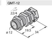
Quick-mount bracket with dead-stop; material: brass, PTFE-coated; Male thread M16 × 1. Note: The switching distance of the proximity switches may change when using quick-mount brackets.
