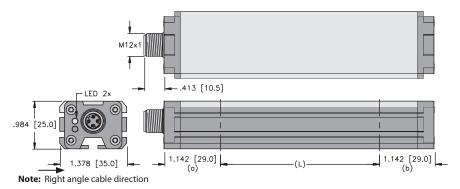
**Ordering Information**The Q-track linear position sensors are available in different lengths from 100 to 2,000 mm, in increments of 100 mm. The sensors, mounting accessories, and positioning elements are available individually or as a kit.
