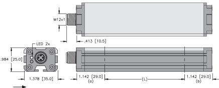
\*Operates at a distance of 0-4 mm from the sensor surface
