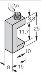
Mounting bracket for mounting magnetic field sensors on tie-rod cylinders; cylinder diameter 32... 63 mm; material: Stainless steel
