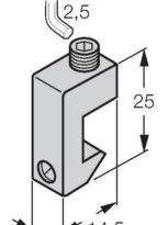
Mounting bracket for mounting magnetic field sensors on tie-rod cylinders; cylinder diameter 32... 50 mm, material: Anodized aluminum
