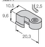
Clamping piece for mounting magnetic field sensors on dovetail groove cylinders; clamping width: 10.5...12.4 mm; material: Aluminum; further mounting accessories for other clamping widths on request
