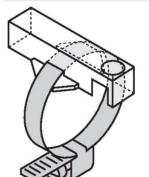
Mounting bracket for mounting magnetic field sensors on round cylinders using tensioning straps; material: Trogamid; please order retaining straps separately
