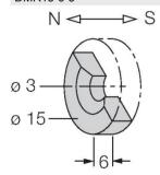
Actuation magnet, Ø 15 mm (Ø 3 mm), h: 6 mm; attainable switching distance 36 mm on BIM-(E)M12 magnetic field sensors or 32 mm on BIM-EG08 magnetic field sensors; for Q25L linear position sensors: recommended distance between the sensor and magnet: 3...4 mm
