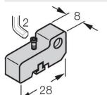
Mounting bracket for mounting magnetic field sensors on SMC cylinders; clamping width 4 mm; material: Anodized aluminum
