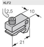
Mounting bracket for mounting magnetic field sensors on profile cylinders (IMI Norgren); cylinder diameter: 32...100 mm; material: Anodized aluminum
