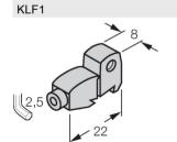
Mounting bracket for mounting magnetic field sensors on profile cylinders with external dovetail guide; for all cylinder diameters, material: Anodized aluminum
