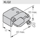
Mounting bracket for mounting magnetic field sensors on profile cylinders; cylinder diameter 50... 100 mm; material: Anodized aluminum; please order mounting bracket separately
