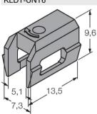
Mounting bracket for mounting magnetic field sensors on dovetail groove cylinders; groove width: 7.35 mm; material: PPS
