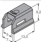
Mounting bracket for mounting magnetic field sensors on dovetail groove cylinders; groove width: 7 mm; material: PPS
