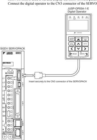
The JUSP-OP05A-1-E optional digital operator for the  $\Sigma$ -V Series SGDV SERVOPACK is used to set and display the SERVOPACK parameters. Connect the digital operator to the CN3 connector of the SERVOPACK.
