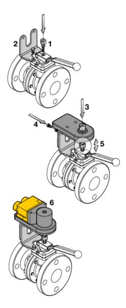
Screw the self-locking nut on the actuator screw and then the actuator screw in the manual valve (1).
