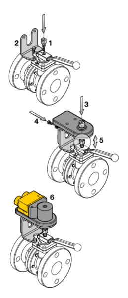
Screw the self-locking nut on the actuator screw and then the actuator screw in the manual valve (1).
