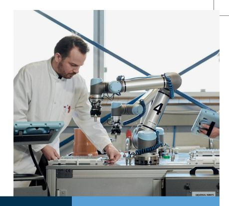
Cobots from Universal Robots can provide easy access to the consistent speed, repeatability and force control essential for a wide range of industrial processes. This enables you to automate and to increase productivity as well as to ensure higher – consistent – levels of quality in key manufacturing processes such as gluing, dispensing, painting, grinding, deburring and polishing.
