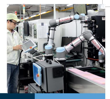
Pick & place operations are one of the automated tasks for which cobots from Universal Robots are most often used. Our cobots are ideal for a wide spectrum of such setups, from those requiring high positioning accuracy to those requiring a vision system to locate the part. The high repeatability provided by UR cobots ensures exceptional accuracy in all kinds of automated pick & place taskings.
