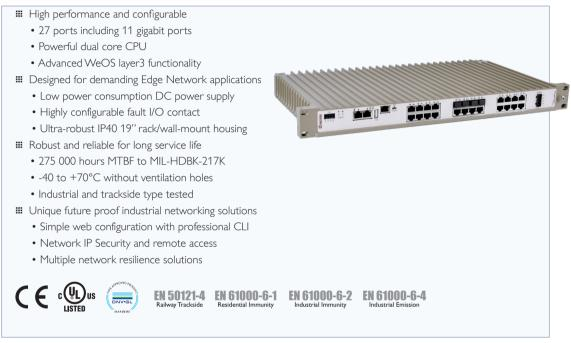
The RFIR (RedFox Industrial Rack) is a high performance layer 3 industrial Ethernet switch designed for high network traffic applications. Various port configurations are available that can be further customised with SFP transceivers. RFIR is powered by the Westermo WeOS network operating system.
