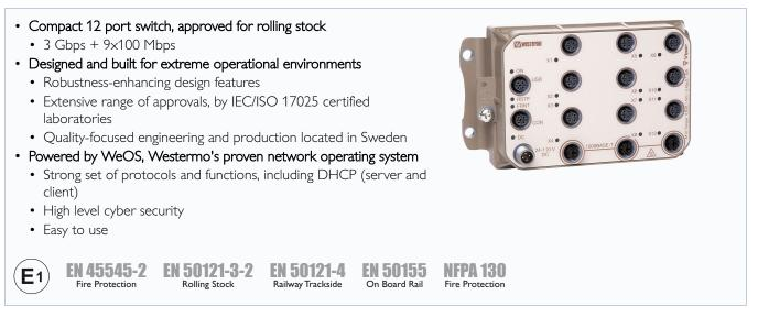
The Viper-112A-T3G is a managed 12 port switch optimised for the needs of the railway rolling stock market. Gbps ports cope with high bandwidth devices such as access points and NVRs (Network Video Recorders).
