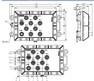
Weight 0.9 kg Degree of protection IP65
